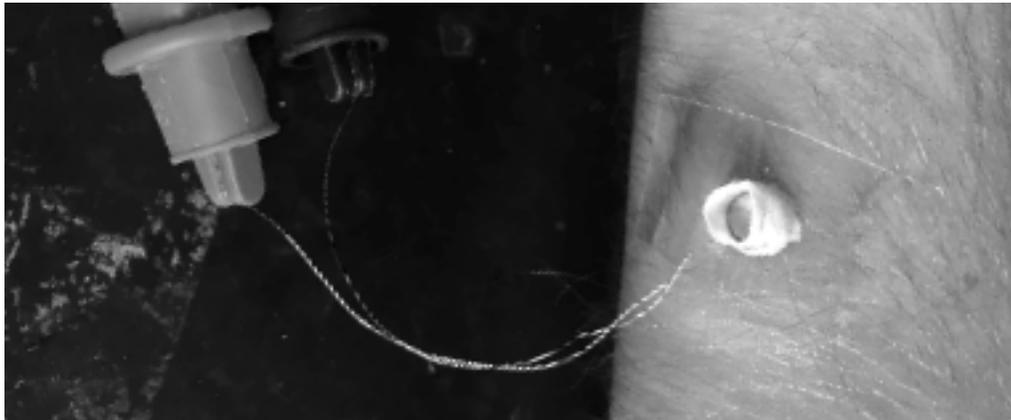
For this reason we had to fallback to the ERM technology that is more conventional and reachable in a short timeframe. So we used coin motors to arise the skin nerves and simulate a pressure.
