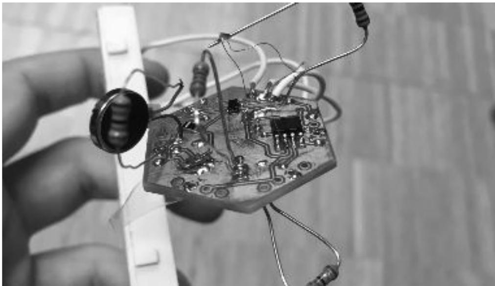
We realized the design with 6 Velostat patterns and pressure points is not the optimal way to get a good value for pressure because the velostat contact traces were connected parallelly and impossible to calibrate individually. Additionally due to the placement of components on both sides the PCB size was too big and also not easy to assemble in a batch process. Therefore, the PCB design was redesigned again.
