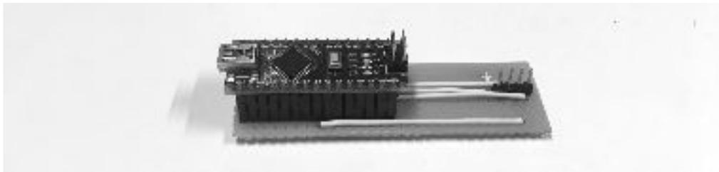
This should eliminate faulty boards that should be integrated into the **eSkin**. During the assembly process, instead of soldering everything together, we decided to make small patches just for several cells and then connect the patches together. The rationale for this is to spot the error at an early stage. Otherwise, we would have to do a “binary search” for the whole setup, thus separating cells and soldering them again, which requires more time and work.
