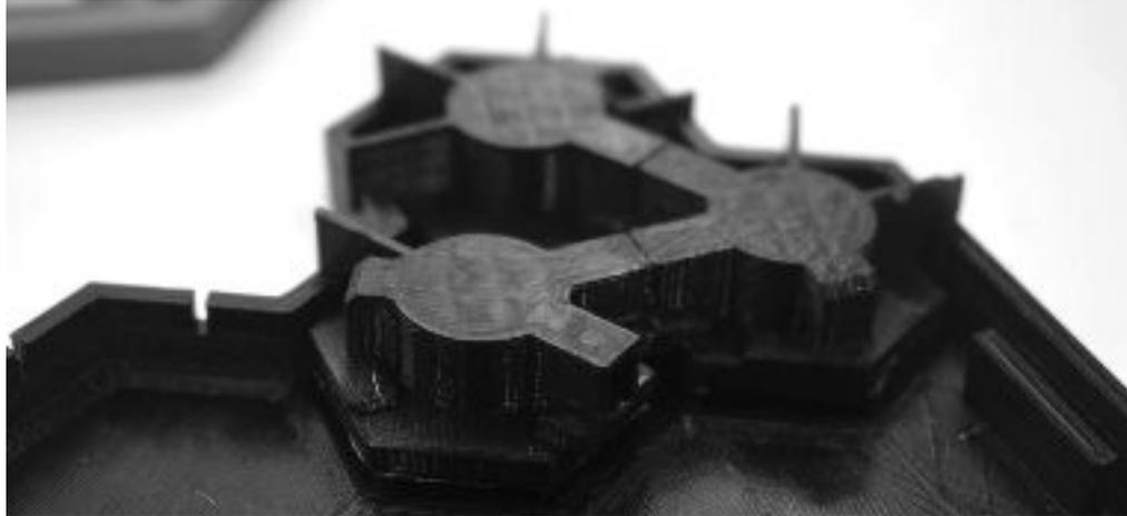
The bridges were cut in half and then had a piece extruded out so it acted similar to a male head while other cells had a hole placed in their bridge half having it act like a female head. This allowed for all of the cells to be joined together securely and hang above the base of the bath while also still being able to remove the filler form from the silicone without breaking it meaning we could produce a large number of silicone patches just from these 2 printed components.
