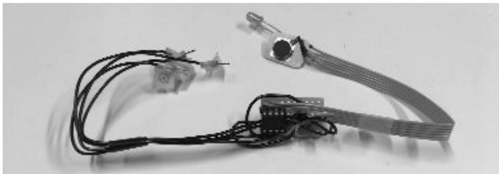
As an evaluation test of this setup the value from the self designed FSR was received over I<sup>2</sup>C by the Arduino Uno MCU, mapped, and sent back to the motor and LED of the same cell.
